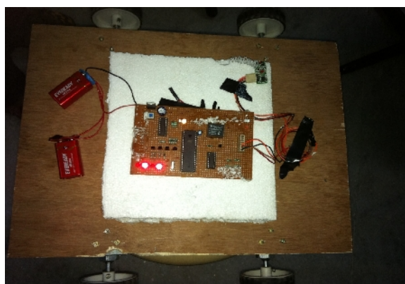
Fig. 17. Digital binary output 0101 shows right turn direction.
